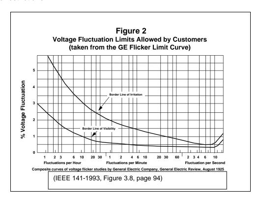
The allowable maximum voltage drop at a motor's terminals or on the Customer's own distribution system depends upon the Customer's requirements. It is the Customer's responsibility to ensure that the starting of their motor does not result in an unacceptable voltage drop within their facility.
